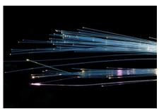
"bouncing" it at just the right angles. The glass acts as a mirror, bouncing the light all the way to my house. The cable has an outer layer of glass called the cladding that keeps the light inside the cable and helps keep the light bouncing and reflecting all the way—with no loss of strength!
